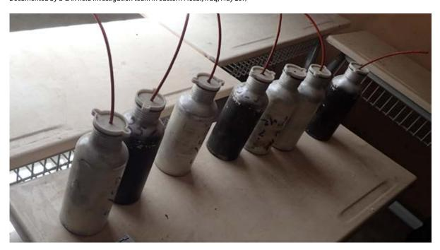
IS forces had pierced the plastic cap of each container to insert a length of safety fuse. When ignited, the safety fuse burns for a predetermined period of time, depending on the length of the fuse. The safety fuses protruding from each of the flasks had been cut to roughly the same length, which suggests that the fuses would burn for approximately the same amount of time before their flames would reach the contents of the container.
