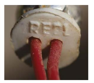
**Figure 194 A non-electric detonator produced in India**Documented by a CAR field investigation team in Kobane,
