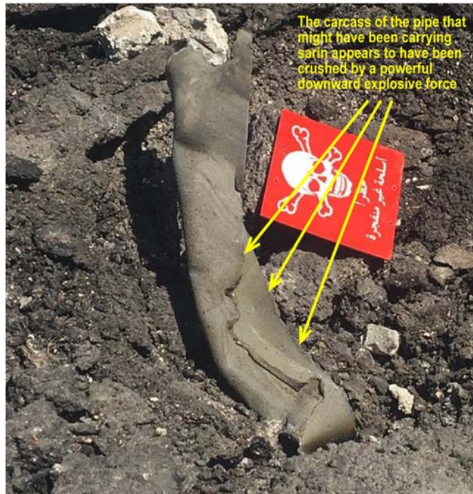
Deformation of sarin containing pipe and crater from the action of the explosive charge placed on top of the sarin containing pipe. Note that pipe has been flattened from the outside and has failed along its length and at the far end due to the action of the incompressible sarin fluid against the pipe walls.
